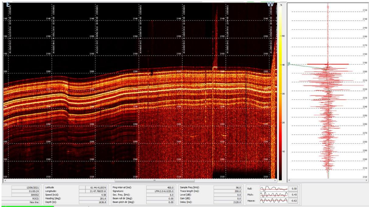
**Fig. A15. Image taken during the break-down of the Topas system (noisy signal starting at 00:43).**
